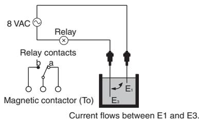
A pump is usually connected to a contactor, which in turn is connected to the Controller contact outputs. The Level Controller would automatically operate the pump, to control the liquid level in the tank.
