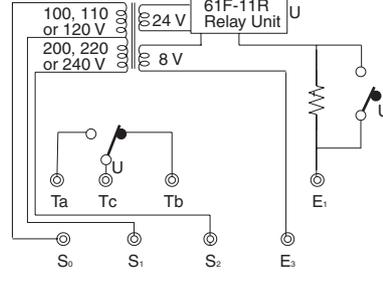
**Note:** The 61F11H relay deenergizes when there is water present across the Electrodes, whereas the 61F relay energizes when there is water present across the Electrodes.
