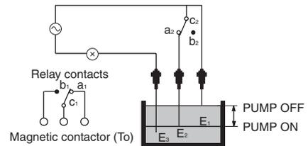
As shown in the above figure, when the holding circuit relay is energized, contact a<sub>2</sub>, its NO contact, is closed. The electrical circuit made through the liquid and the electrodes is then retained by E2 and E3, even when the liquid level falls below E1, as long as contact a<sub>2</sub> is closed.
