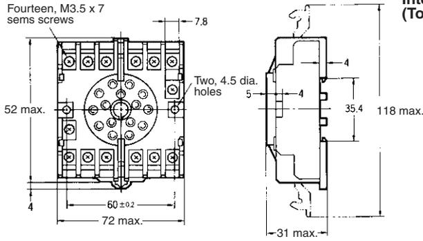
M3.5 x 11.5 sems screws for terminal screws
