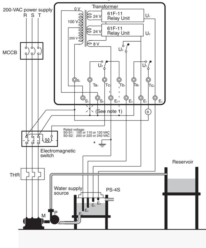
**Note: 1.** The diagram shows the connections for the water supply. When draining, change the connection from terminal Tb1 to terminal Ta1.
