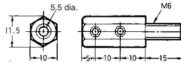
**F03-07 U-shaped Electrode Band Weight (SUS304)**
