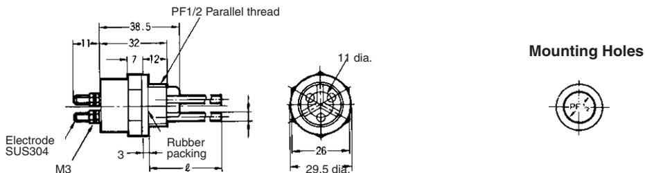
**Note:** Standard holder construction includes three integral 300-mm-long Electrodes. However, a model having 1,000-mm-long Electrodes is available on request.
