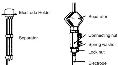
When the required length of Electrode is more than 1 m, use a Separator at each joint of two Electrodes so as to prevent the Electrodes from contacting one another.
