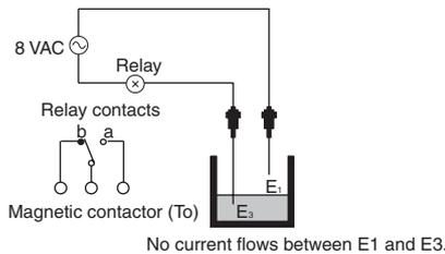
When electrode E1 is not in contact with the conductive liquid, the electrical circuit is open, and no current flows between electrodes E1 and E3.
