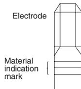
5. When long Electrodes are required, connect them with connecting nuts and lock nuts (2 pieces) every 1 m.
