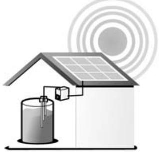
Liquid level control for remote regions without AC power supply.
