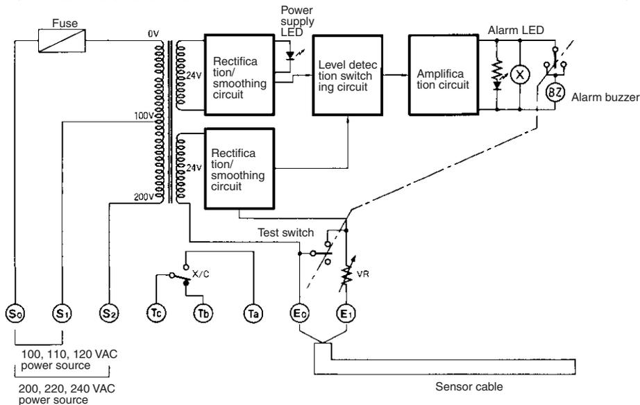
61F-GPN-V50 Water Leak Detector
