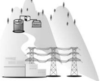
Cut costs by using the 61F in situations where ultrasonic/electrostatic capacity level controllers were used because only DC power supply was available.
