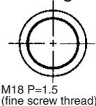
\*This nut is made of Fluoroplastic
