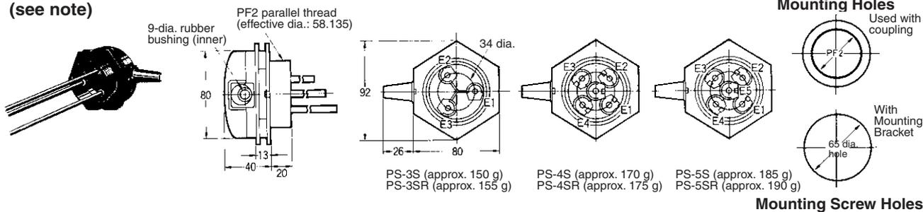
**Note:** The PS-3SR, PS-4SR, and PS-5SR have built-in resistor of 6.8 kΩ and used for the two-wire 61F models.
