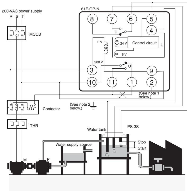
**Note:** 1. The diagram shows the connections for the water supply. When draining, change the connection from terminal 1 to terminal 11.
