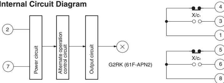
Connect the output terminal Ta of the 61FG□ to input terminal 2 of the 61F-APN2.
