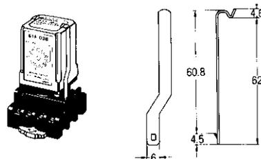
To mount the 61F-03B/-04B Unit to the PL11 Back-connecting Socket, use the PLC-1 Mounting Brackets.
