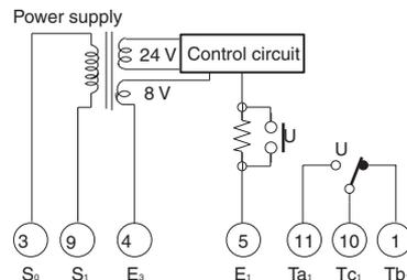
**Note:** When applying a self-holding circuit, short between terminals 5 and 6 and use terminal 7 as E<sub>2</sub>.
