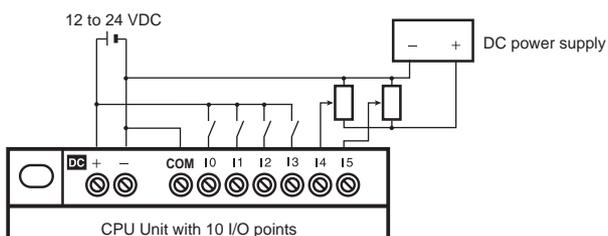
**Note:** When connecting an analog input device, always connect the negative side to the COM terminal.
