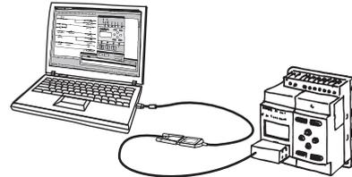
**Note:** For notebook computers that do not have an RS-232C serial port, connect the computer to the ZEN by connecting an OMRON CS1W-CIF31 USB-Serial Conversion Cable to the ZEN-CIF01 Connecting Cable.
