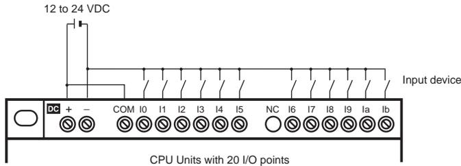
**Note:** When connected to the positive (+) common, Ia and Ib cannot be used as analog inputs.
