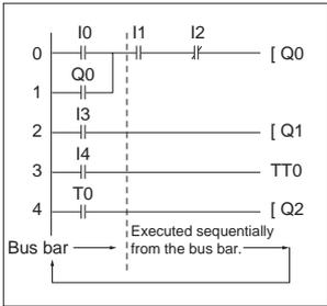
ZEN executes the entire ladder program (up to 96 lines) from the first to last line at one time. Each row is executed in order from left to right starting from the left bus bar.
