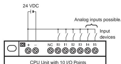
**Note:** I4 and I5 (Ia and Ib for CPU Units with 20 I/O points) cannot be used as analog input terminals.
