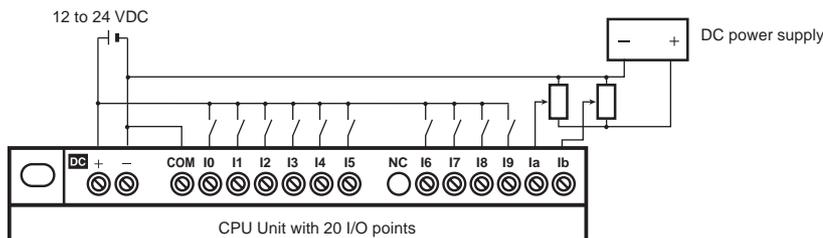
**Note:** When connecting an analog input device, always connect the negative side to the COM terminal.
