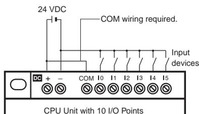
The input circuit common terminal is connected internally to the negative (-) side of the power supply circuit.
