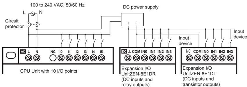
**Note:** When connecting Expansion I/O Units with DC inputs to a CPU Unit with an AC power supply, the burst noise immunity will be 1 kV (IEC 61000-4-4).
